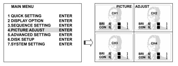
You can use the "^" and "v" buttons to adjust the **BRI** (brightness) and **CON** (contrast) properties of the live images in each channel.
